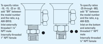
Drive inlet and exhaust are ½" NPT female. Drive inlet also includes a ½" NPT male x ½" NPSM female (straight pipe thread) swivel adapter (connecting male nipple should include 30° inside bevel for proper fit).
